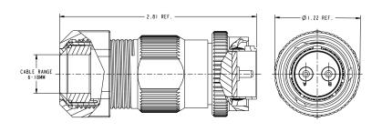
C10-694782-03P 3 WAY 400VDC/250V AC MALE PANEL RECEPTACLE IEC61984 Certified
