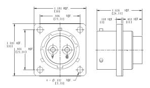
C10-694780-02S 2 WAY 48 VDC FEMALE STRAIGHT PLUG IEC61984 & IEC60950-22 Certified
