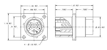
C10-694782-03S 3 WAY 400VDC/250V AC STRAIGHT PLUG IEC61984 Certified
