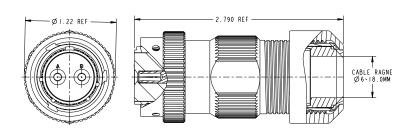
C10-694781-02P 2 WAY 48 VDC MALE STRAIGHT PLUG IEC61984 & IEC60950-22 Certified
