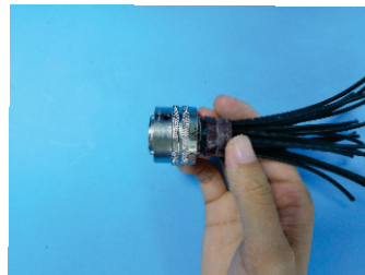
8. Re-check to make sure the grommet is against the insulator face after all contacts are seated
