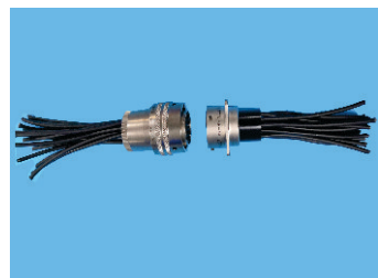
12. Thread and tighten backshell then unmate from receptacle
