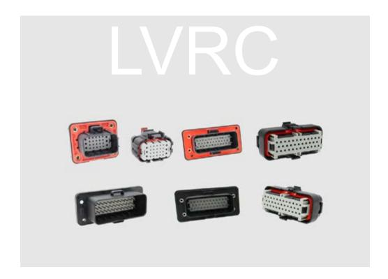
Low Voltage Rectangular Connectors light weight, multiple coding positions, 26 & 35 position low voltage available, also we provide 12 position high voltage connectors are designed to meet USCAR-2, USCAR-37 specifications. With a current carrying up to 13A, 250V and 12 position up to 800V, the LVRC connectors can be used in many hybrid and electric vehicle device applications.
