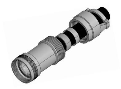
These Backshells from Amphenol not only provide the cable support and strain relief, but ensure the cable sealing and environment protection by means of high quality sealing grommet and grommet follower. The strain relief nut is tightened squeezing the grommet on to the cable jacket during assembly. These Backshells from Amphenol give 6 feet water sealing protection when used with perfectly jacketed cable and are suitable for harsh environment applications.
