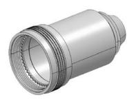
This style is same as that of Spin Coupling with the additional feature of 'self locking'. The free movement of the coupling nut is arrested by suitable device so that the accidental de-coupling is prevented within the specified vibration levels.
