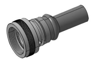
This adaptor is supplied with some length of braid attached. This braid overlaps with the cable braid and effective shielding takes place due to its 360° contact. It is designed to accept heat shrink boot. Ease and less time for cable termination are the prime advantages here.
