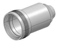
The coupling nut is captivated in the Backshell follower by suitable retention mechanism. This style facilitates the free rotation of the coupling nut and hence assembly of Backshell to the connector becomes easy without turning the entire Backshell body. Lock wire holes are provided on the coupling nut to prevent accidental decoupling when specified.
