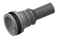
This adaptor is supplied with some length of braid attached. This braid overlaps with the cable braid and effective shielding takes place due to its  $360^{\circ}$  contact. It is designed to accept heat shrink boot. Ease and less time for cable termination are the prime advantages here.
