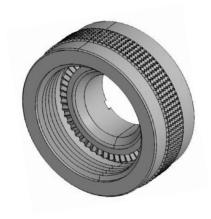
Amphenol Back Nut provide a good grommet-holding force for the crimp Connector, when expensive and heavy back shells are not used. Such holding force is essential to hold the contacts and grommet in place when terminated with wire bundles.
