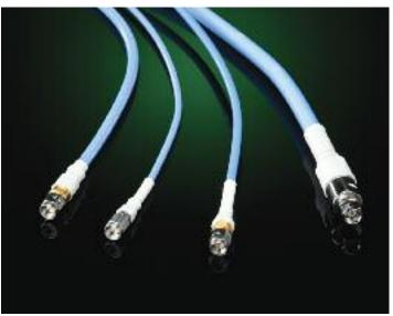
PhaseTrack® cable assemblies are designed for applications demanding minimal phase change over temperature. All PhaseTrack cables use proprietary  $TF4^{TM}$  dielectric that does not have the abrupt shift in the phase that occurs with solid or tape wrapped PTFE based products under normal room ambient temperature conditions.
