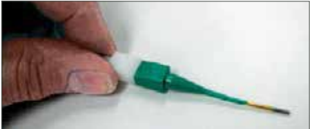
Plastic tool with contact in proper position.
