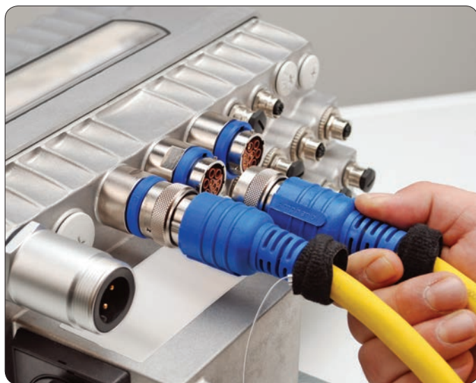
Color-coded thermoplastic bands for visual verification.
