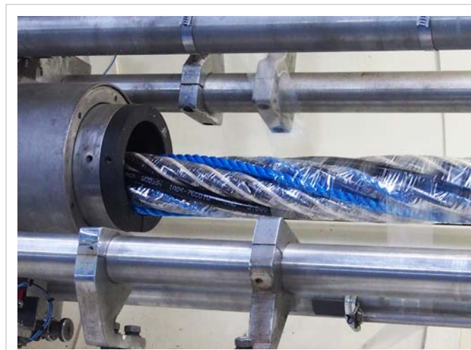
Twisted hose, cable, rope bundle / extruded polymer sheathing
