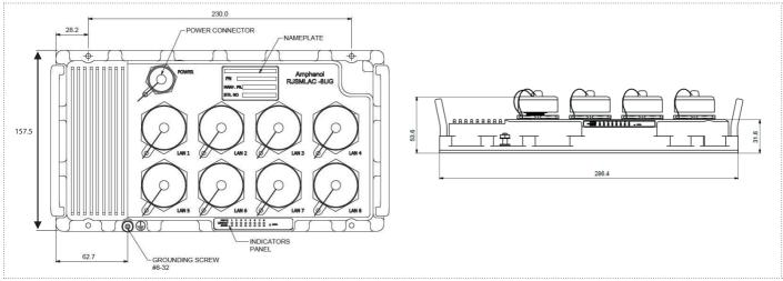
Dimensional line drawing - All measurements are in millimeters
