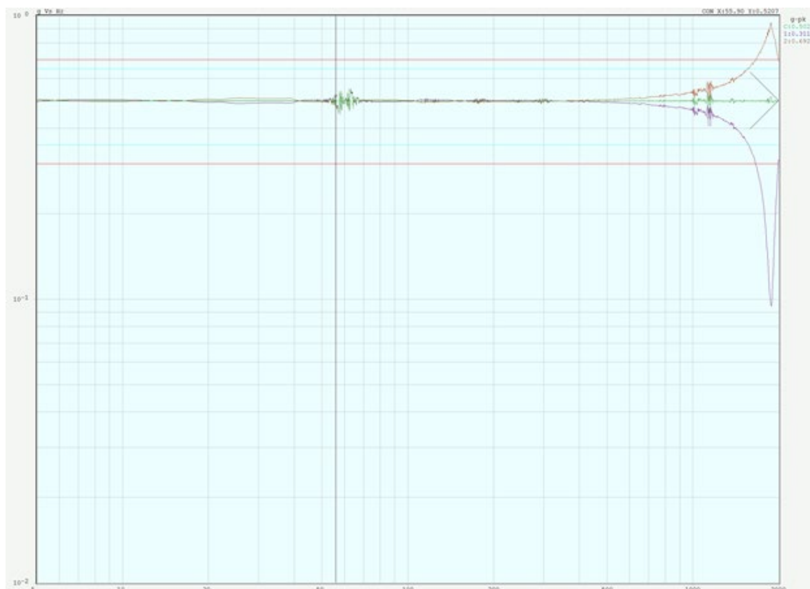
Y axis sine sweep bare fixture
