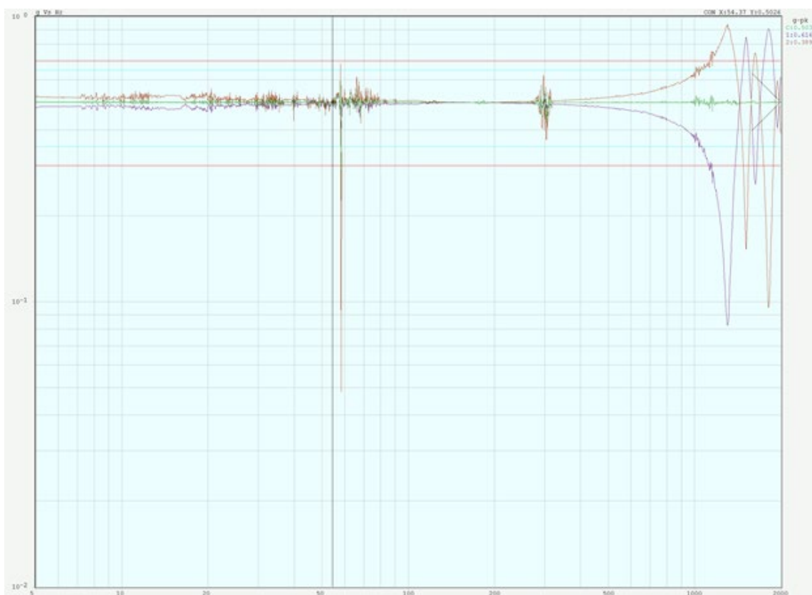
Y axis sine sweep with fixture back plane and cables
