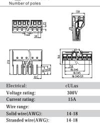
Wire strip length: Withstanding Voltage:
