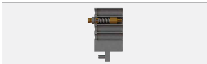
Figure 10.3 Final Assembly. Connector Module + Contact + Bullet
