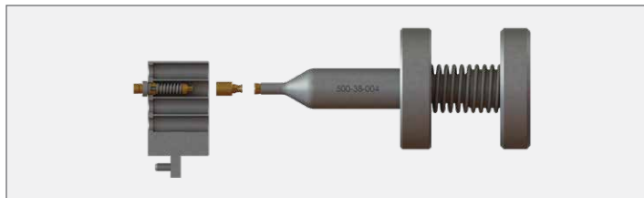
Figure 10.1 Bullet Installation to Contact. Uses Tool PN 500-38-004.
