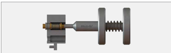
Figure 9.4 Bullet Removed From Contact. Uses Tool PN 500-32-007.
