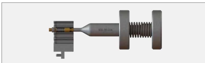
Figure 10.2 Bullet Fully Seated in Contact
