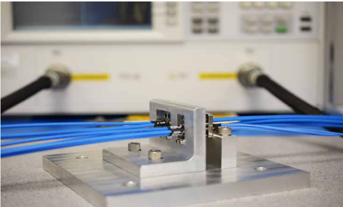
Figure 3 Test Setup for Mated Pair VITA 67.3 SMPS
