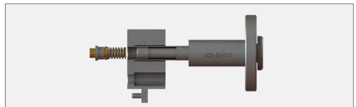
Figure 9.7 Contact Removed from Block
