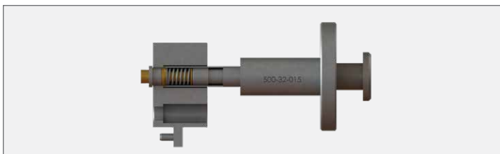
Figure 9.6 Contact Removed. Uses Tool PN 500-32-015.
