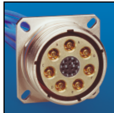
Special Hybrid Ground Plane Connector* with a standard MIL-DTL-38999 insert surrounded by a metal ground plane insert. This connector is designed for applications where the twinax contacts are required to be electrically bonded to a common ground while insulated M39029 signal or power contacts are also included for compact packaging.
